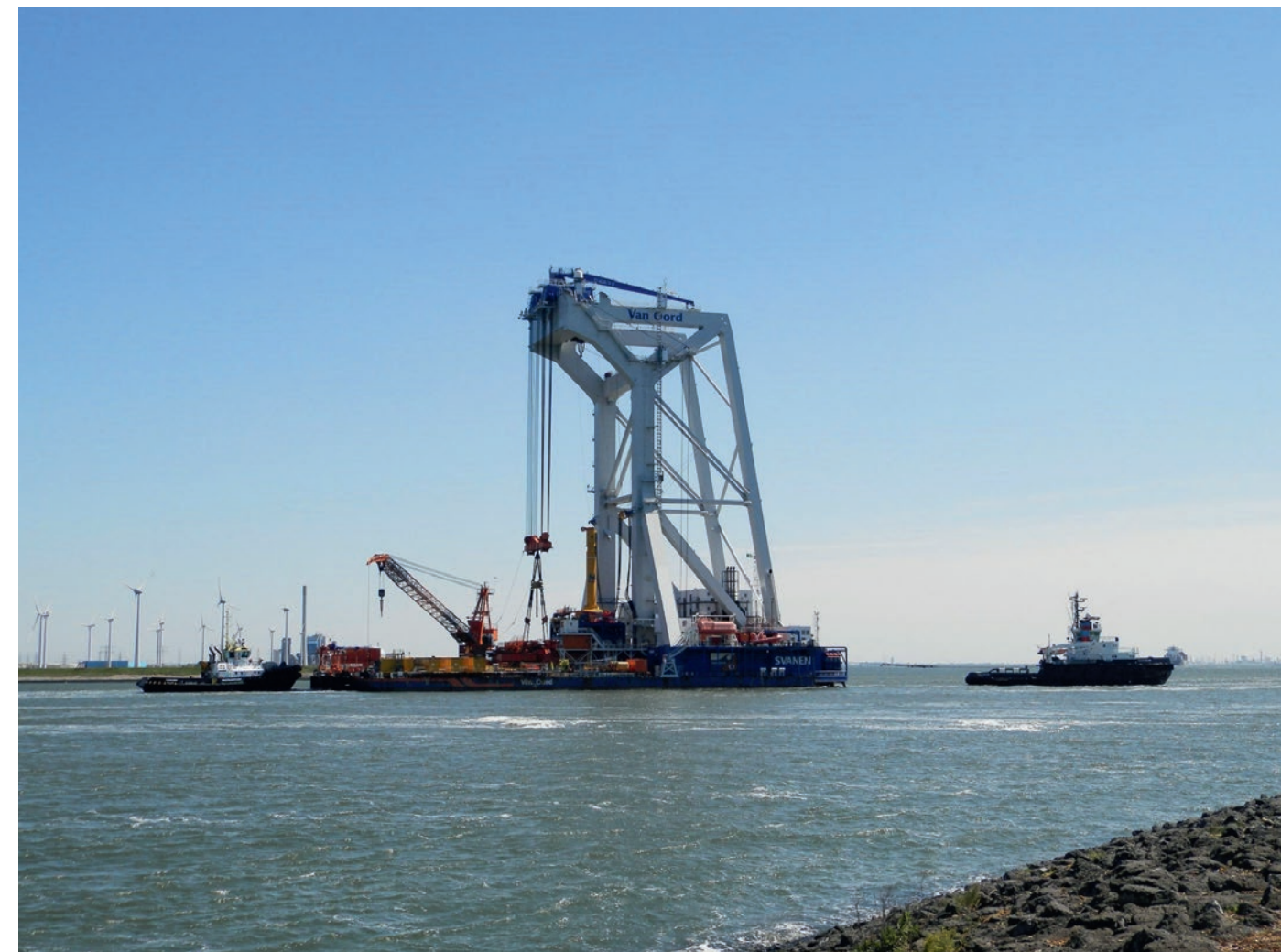
▲ Zeus of Finland towing the heavy lift installation vessel Svanen from Vlissingen to the Kriegers Flak Offshore Wind Farm.
